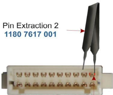
Insert the tips into **red areas** and press down to release pin
